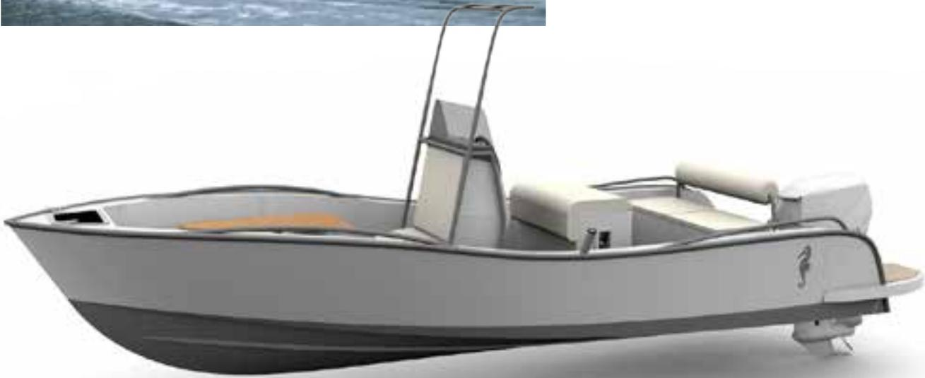
"The hull is fully welded with double pulsed arc welder "weco power pulse" , with continuous alloy thread ALM G 5.
